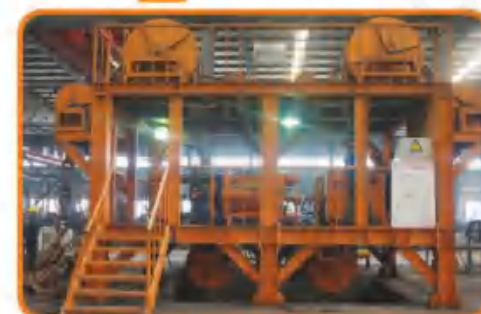
↓ 横档压延 (系泊链) Stud Expansion (Offshore Mooring Chain)
